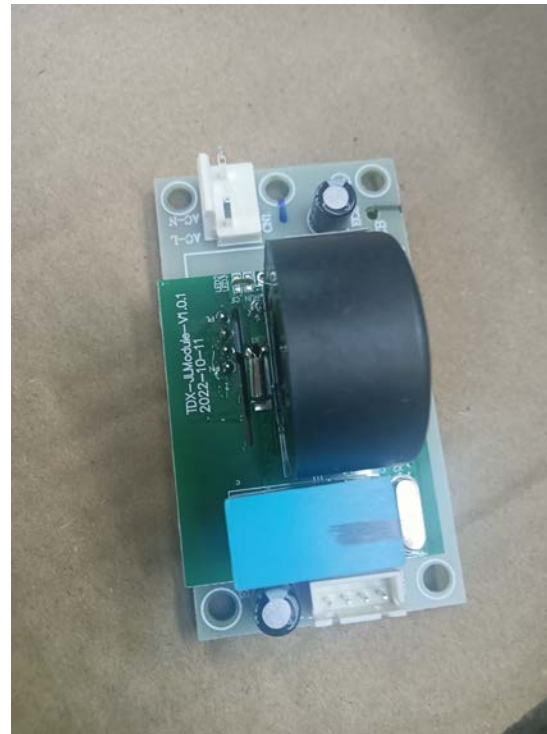
Single-phase metering board
