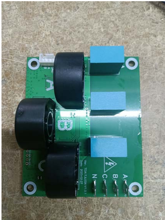
Three-phase metering board
